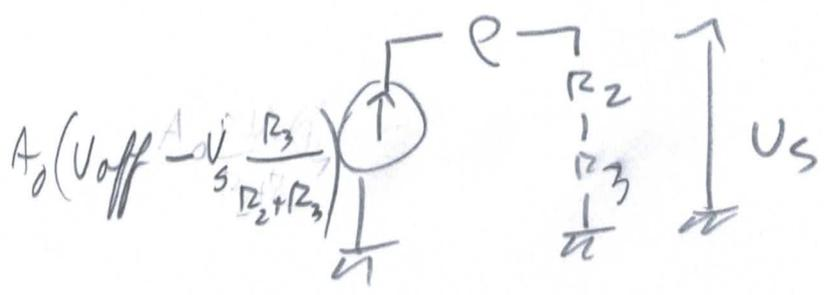
$$U_s = \frac{R_2 + R_3}{R_2 + R_1 + R_2} A_0 \left[ U_{off} - U_s \frac{R_3}{R_2 + R_3} \right] \quad R_2 \gg R_3$$
